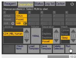
Figure 6.4: A cell separation using CD4 MicroBeads, human will be performed on sample positions 1 and 2. After processing sample 2 the "Sleep" program will be performed as a final wash step before the instrument goes into sleep mode. Clicking "Run" will start the experiment.
