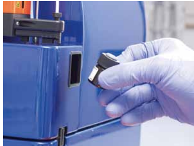
Figure 5.3: The optimal reading distance is 0.5–2.5 cm from the code reader cover, tilt the vial as shown above.
